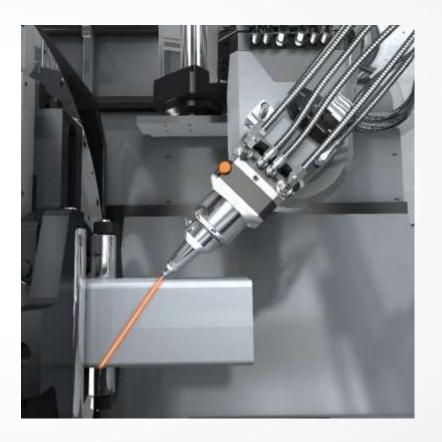
It can realize the bevel cutting ability of the pipe end face, and the pipe can be seamlessly spliced
