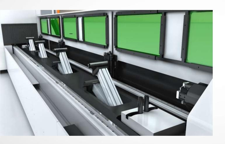
Rolling support, avoid tube sagging while cutting small tube and heavy tube; Follow support, the support frame rises and falls automatically with the rotation of the pipe to avoid scratch of the tube surface; **Concave wheel centering structure to prevent** tube deflection, to avoid collision betwenn tube and chuck.
